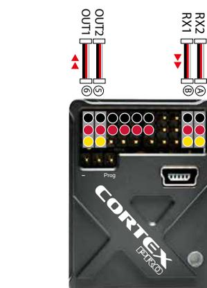
Depending on the receiver or power/servo distribution box, the CORTEXpro handles up to 16 stabilized channels, up to 24 channels all together. All channels that are subject to being stabilized must be programmed to the lowest 16 channels per assignment in the transmitter. All channels from 17 to 24 will only be run through without stabilization. Same for ones in the low 16 channels, which are not moved during teach-in. Thus, these can be used as „normal“ channels too.
