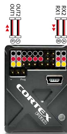
Connect one receiver to port A, or, respectively, two receivers to the ports A and B. Ports 5 and 6 output the serial protocol, which can be used for either one or two inputs into a distribution box.
