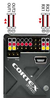
Depending on the receiver or power/servo distribution box, the CORTEXpro handles up to 16 stabilized channels, up to 24 channels all together. All channels that are subject to being stabilized must be programmed to the lowest 16 channels per assignment in the transmitter. All channels from 17 to 24 will only be run through without stabilization. Same for ones in the low 16 channels, which are not moved during teach-in. Thus, these can be used as „normal“ channels too.
